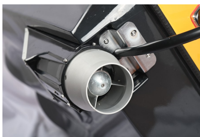
Brushless waterjet propulsion unit
