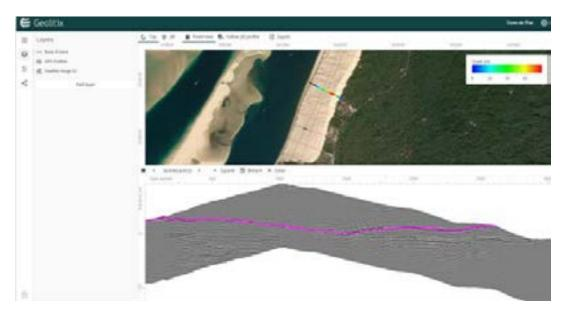
Geolitix offers powerful tools for interpreting your data, enabling you to define 3D points, horizons, or polylines for pipes and cables, as well as vectorised drawings. Each of these layers can be re-ordered in the manner of GIS software, as well as exported in a variety of georeferenced formats.
