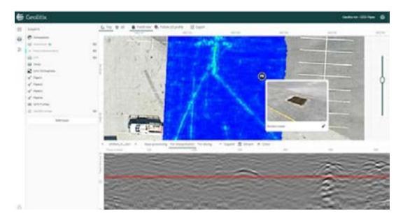
Photos and notes taken in the field are invaluable for later interpretation of subsurface data. Photos taken with GPS-enabled phones and cameras are automatically placed in the correct position on your project space.
