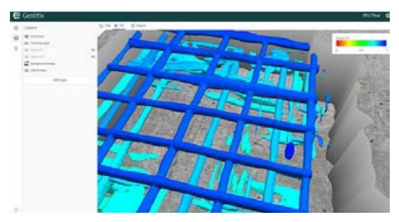
For some applications, such as rebar or void mapping, you may need to create a 3D model of a radar target. Geolitix can easily create 3D isosurface models from GPR profiles for a better understanding of discrete targets.
