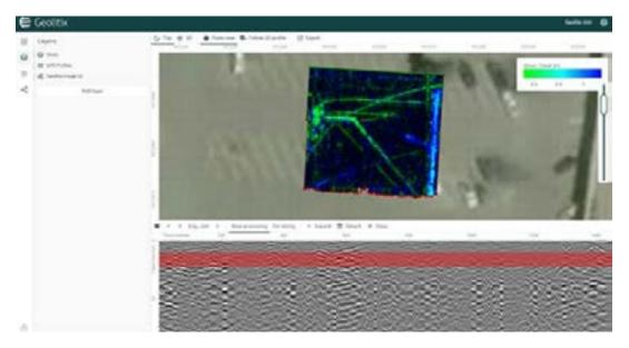
Geolitix allows you to slice your 3D or multichannel GPR data with a few clicks. Complex parameters are suggested for you, allowing you to focus on data analysis.
