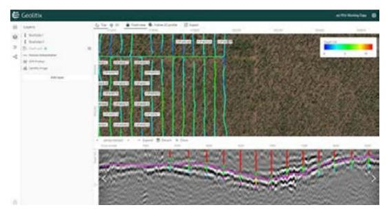
Drilling and coring data can be imported to assist in data interpretation. Geolitix displays lithologies with colour codes and multiple assay results. Drilling data are automatically projected onto the nearest subsurface profiles within a user-specified distance.
