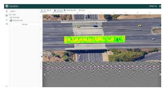
Rebar corrosion and pavement delamination can be visualised by mapping GPR reflection amplitudes. Geolitix generates these maps in seconds—there's no need to perform calculations or import data into other software.
