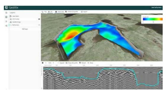
Creating 3D surfaces of geological layers or thicknesses is easy with Geolitix. Simply select the interpreted layers you want to map and the gridding parameters are automatically calculated for you.
