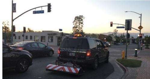
Figure 1, Typical environment in which GPR-Array data is gathered
