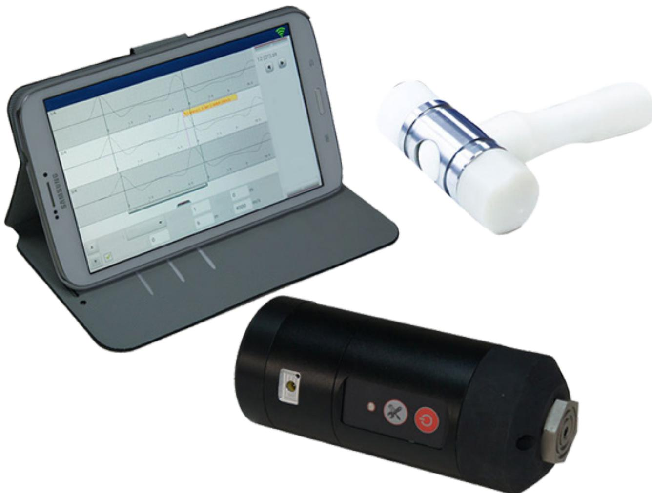
By using the reflected wave method, the instrument is used to **assess the integrity of concrete pile and identify the extent and location of the pile defect.** It can be used for testing drilled piles and hammer piles. It can also be used for testing the exposed top surface of constructions such as pillars.
