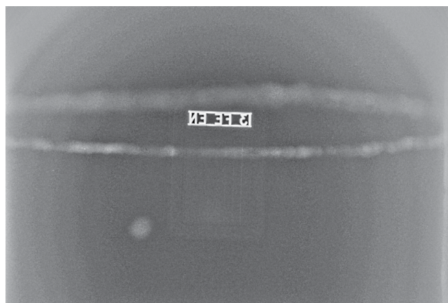
8" Pipe, 2mmx2 Wall thickness, Contact (minimum water)
